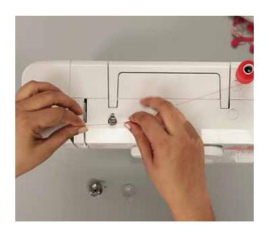
Now we learn how to Thread The machine Raise the thread take-up lever to its highest position by turning the balance wheel towards you.
